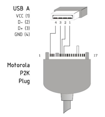
\* Shorted pins 13 and 14 force the phone to enter boot mode. Remove battery, connect cable, insert battery, power the phone ON.
